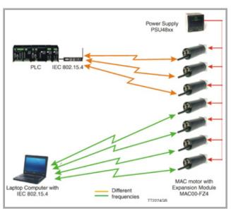
Example of simultaneous communications to two groups of MACOO-FZ4 enabled motors from a PLC and a PC using two different radio channels. With the standard software, one motor in each group is connected to its master controller at any time. With expanded software, all motors in a group can be addressed simultaneously.
